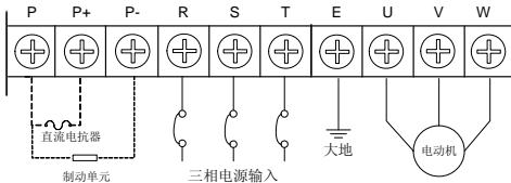
**VII类主回路端子** 适用机型: V560-4T0370 ~ V560-4T0450
